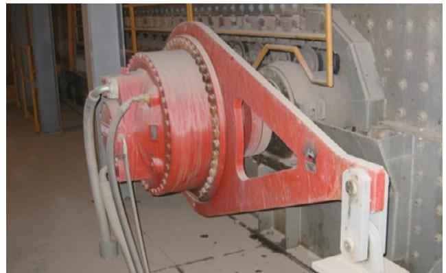
The overhang weight mounted on the head shaft is normally smaller than electro-mechanical torque arm-mounted drives.
