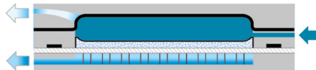
FIGURE 4. Wash water enters the chamber, washing out impurities as it passes through the filter cake before exiting through the filter cloth.
