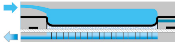
FIGURE 3. The pressing medium enters and squeezes the cake, forcing more liquid out.
