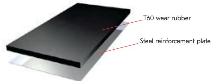
Offers excellent wear resistance in applications with both impact and sliding wear. The steel backing prevents small particles from getting beneath the lining and ensures secure fixing. Rubber wear plates also reduce noise and vibrations while being significantly lighter than conventional steel linings.
