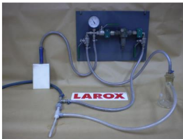
CC Test Kit (Capillary Ceramec Vacuum Filtration)
