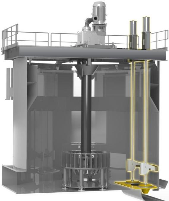
Accurate and reliable level control is one of the key operating variables in flotation. Especially in big cells, every minute of lost concentrate mass pull is worth a considerable amount of money
