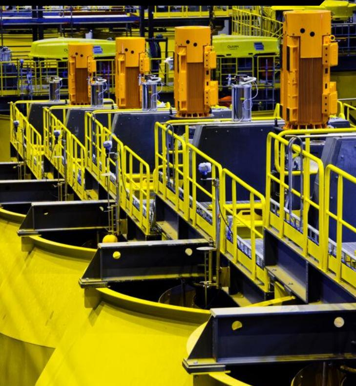
Enhance your flotation cell with an automatic air control system that stabilizes the airflow and provides a faster, more accurate tool for varying the airflow to the cell. [Read more here »](#)
