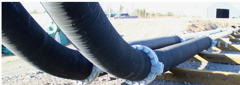
Picture 6: Swivel hoses in tailing application.
