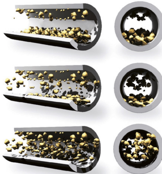
Figure 2: Relationship between different flow conditions and friction losses
