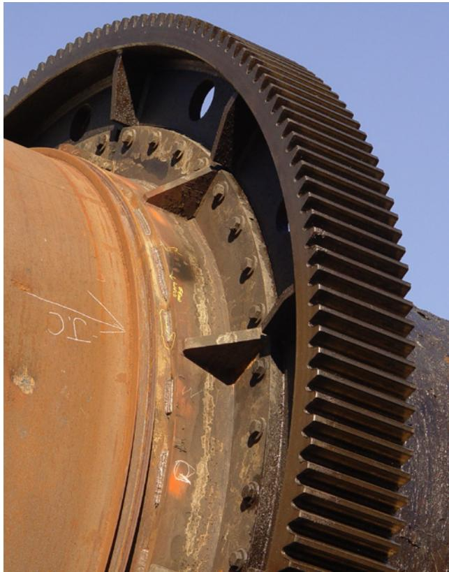
Gear axial runout and radial runout refer to the misalignment of the main gear as it rotates. Radial run-out is checked to ensure proper alignment between the gear and the pinion, while the axial runout is important to ensure proper face contact between the gear and pinion.
