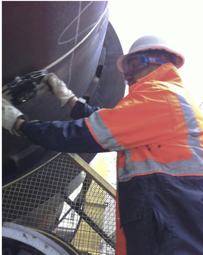
Shell flex or ovality occurs at each pier. This condition is marked by a radial irregularity or deviation from the circular shape at the horizontal axis, and an assumed equal and opposite deviation at the vertical axis.
