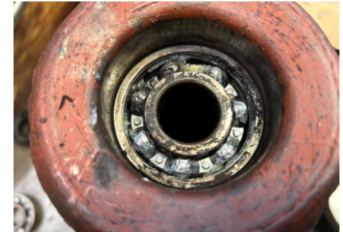
April 12: RollerSense senses a fault — bearing failure
