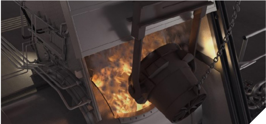
Excellent gas capturing during charging of matte
