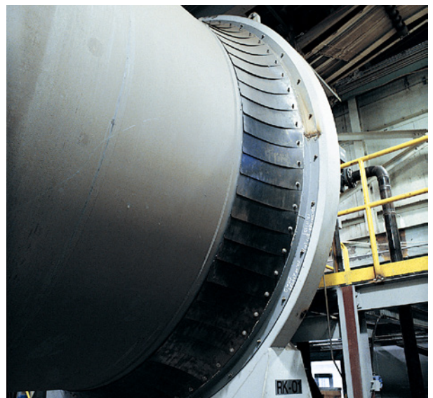
Figure 32: Metso patented leaf seals
