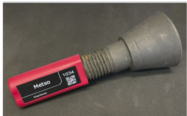
Wear sensor integrated into an M30 TaperLock used to install cast liners in a coarse ore stockpile hopper.
